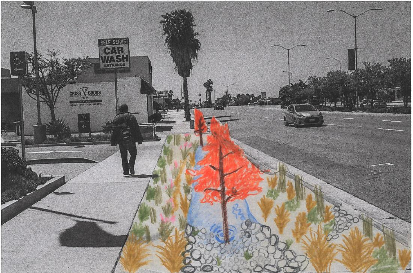
Bioswales collect pollutants and rainwater. Illustration: Brittany Cabeje.
